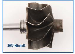
cost, many standard Chinese aftermarket turbine wheels use a Chinese grade alloy which only has either 30% - or sometimes as low as 15% Nickel. You cannot visually tell the difference between these parts. In Chinese engines, these turbos may last as long as expected - but try putting these parts into a European turbo and the result is a warranty failure.
